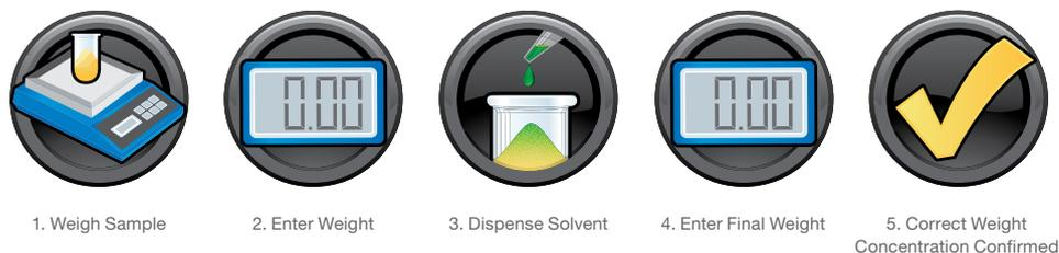
The diagram above depicts how the Microlab 600 Dry Weight Dilution Wizard functions. After the desired concentration and final volume are selected, the instrument then specifies the amount of sample that is required.
