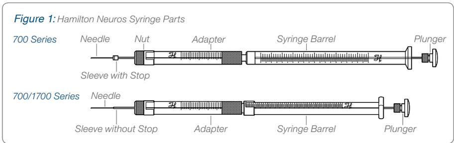
The plunger on a 7000 series syringe is a small tungsten wire that runs to the tip of the needle. The needle and plunger is a match set and cannot be replaced if damaged. Do not pull the plunger completely out of the 7000 series syringe as this will expose the small tungsten plunger wire and will most likely result in irreparable damage.
